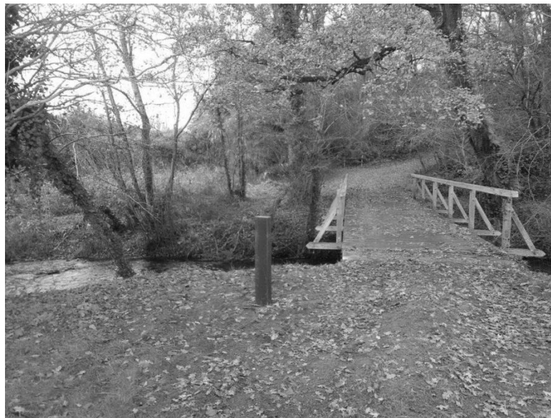
Fig.1 Pedestrian counter installed on a natural trail.
