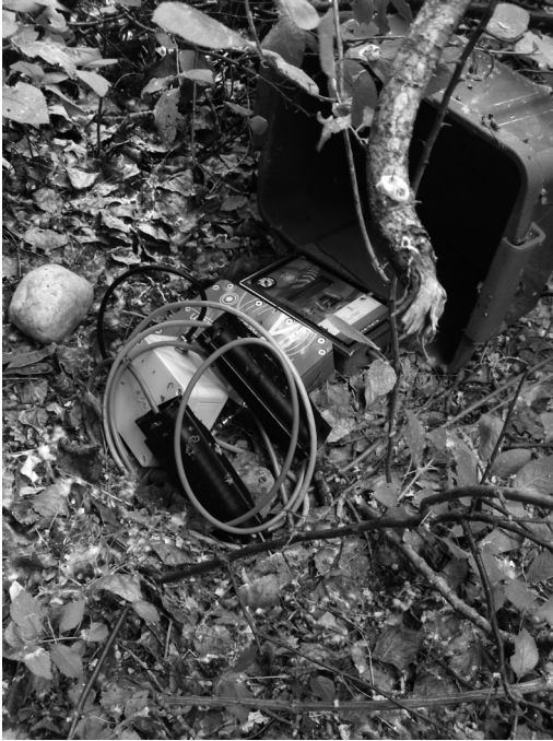
Fig. 1. The Eco-counter - Ecotwin© with the remote control facility (Eco-GSM-unit)
