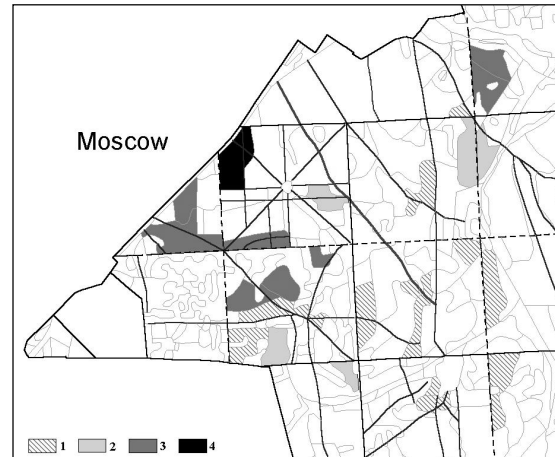
Figure 3. Soil compaction, kg/cm 2 : (1) 1.0-2.0, (2) 2.0-2.5, (3) 2.5-3.0, and (4) >3.0
