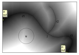
Figure 3a. Cost-Distance function applied on Figure 1, with two entrances used as sources.
